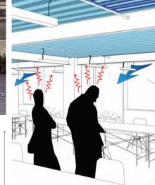
The exposed, radiant-chilled ceilings provide comfort conditions by absorbing heat given out by people and computers
